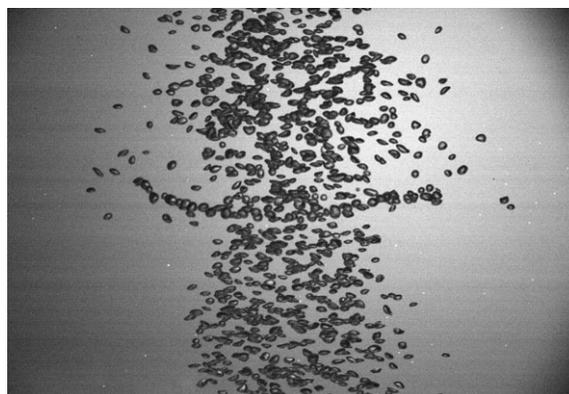
Fig. 10. Perfectly aligned bubbles in a bubble ring.
